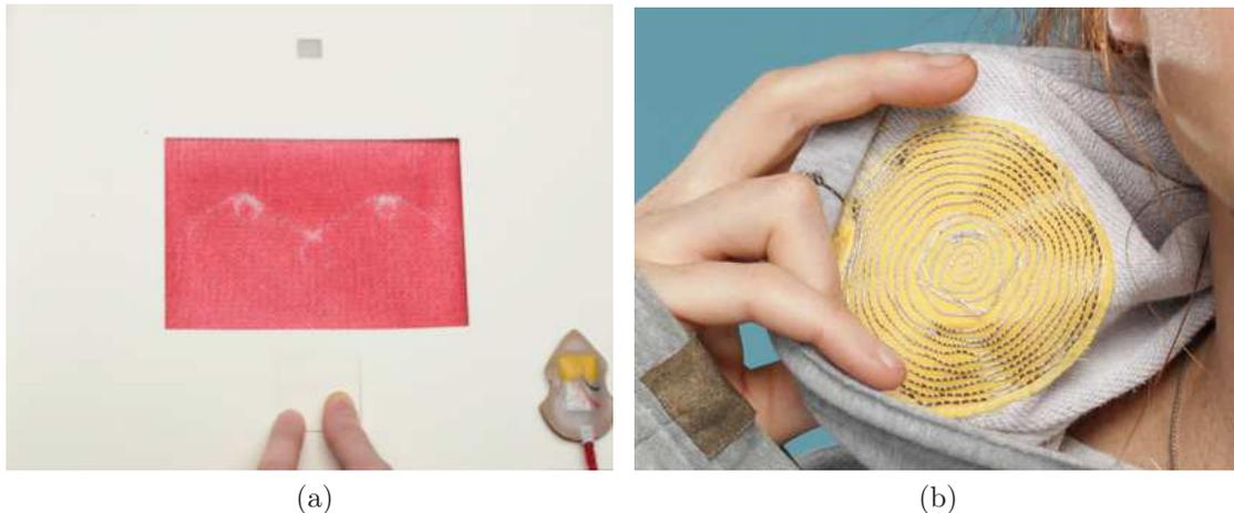
Figure 2.12: Textile output devices: a) Textile thermochromic display and b) textile speaker. Reprinted with permission of Katharina Bredies.
