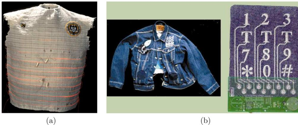
Figure 2.5: a) Georgia Tech's Wearable Motherboard (GTWM) [95]. Copyright ©2002 by ACM, Inc. Reprinted with permission of ACM, Inc. b) *Musical Jacket* [99]. Reprinted with permission of Maggie Orth.
